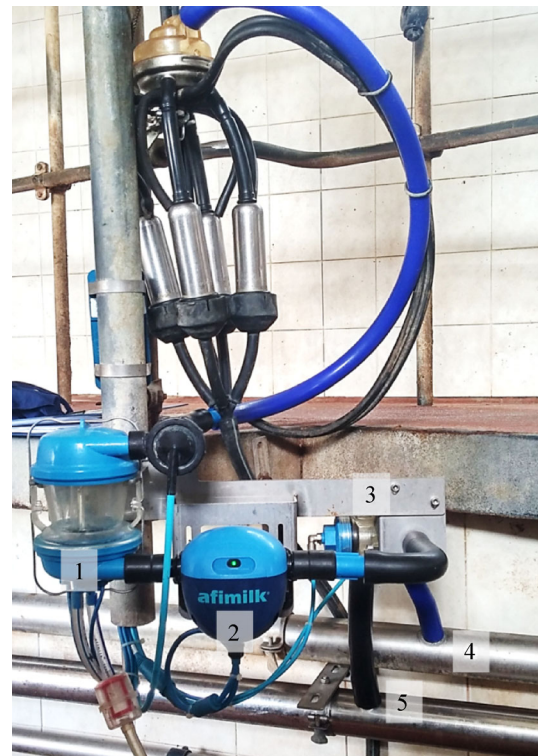
Fig. 1 The AfiLab (2) installed next to the AfiMilk milk meter (1) performs real-time analysis of milk components using spectroscopy in the near infrared. Milk with predefined coagulation properties is separated and channeled using specific valves (3) through two different milklines (4 or 5) in a predetermined refrigeration tank.
