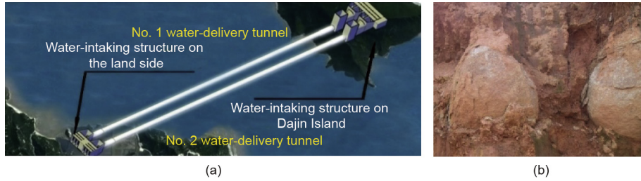
Fig. 10. (a) A sketch of the water-delivery tunnel for the Taishan Nuclear Power Station; (b) locally encountered spherical granite boulders.
