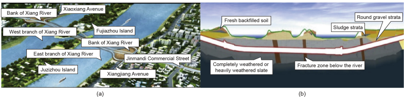
Fig. 7. (a) The plan layout and (b) the profile of Yingpan Road Xiang River-Crossing Tunnel in Changsha.
