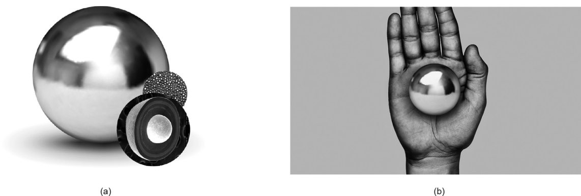
Fig. 1. (a) The large sphere (back (a)) is a pebble studded with thousands of particles of TRISO. The cut-away image (front (a)) shows the multilayer structure of an individual particle, with protective layers of pyrolytic carbon, silicon carbide, and carbon buffer covering a nugget of uranium oxide or uranium oxycarbide. (b) The image indicates the size of a single pebble. Credit: X-energy (public domain).
