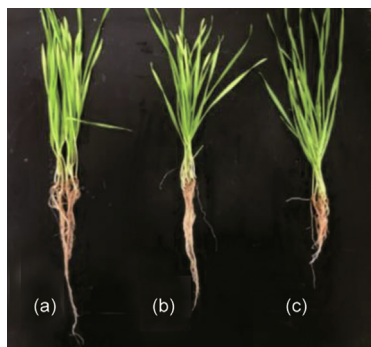
Fig. 12. Growth status of wheat roots in a range of drilling base fluids: (a) No. I; (b) No. IV; (c) No. III.
