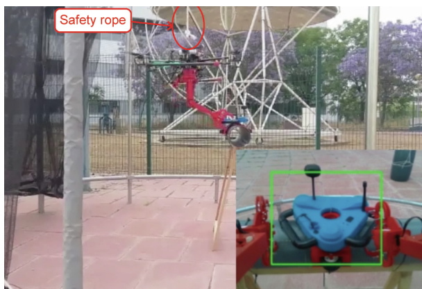
Fig. 16. Outdoor autonomous test with a safety rope.
