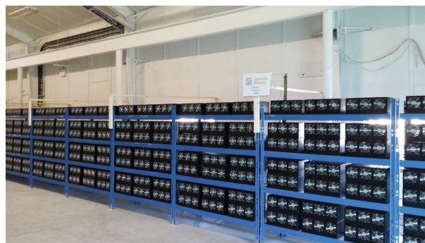
Fig. 1. The cryptographic problems needed to process blocks of cryptocurrency transactions are so difficult they have to be solved by trial and error, often by specialized computer systems, known as mining rigs, that may be deployed in banks of thousands of machines, like these in a cryptocurrency mining farm in Iceland. The energy consumption of this computing activity is substantial, estimated by some studies to equal that of entire countries. Credit: Marco Krohn, Wikimedia Commons (CC BY-SA 4.0).
