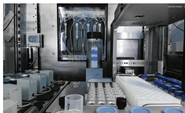
Fig. 1. A snapshot of a live view of IBM's RoboRXN for Chemistry system synthesizing a molecule. On the lower-left quadrant of the picture, some of the automated-synthesis workstation's six reaction chambers are visible. Phials containing ingredients are on the right, with blue caps. Credit: IBM RoboRXN for Chemistry, with permission.
