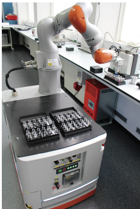
Fig. 2. The “automated researcher” in action at the Cooper Group laboratory at the University of Liverpool, Liverpool, UK. The KUKA Mobile Robot moves freely and has a reach of 82 cm. It identifies its relative position using a combination of laser scanning and touch feedback for fine positioning. It moves slowly, for safety reasons, but the system’s experimental throughput is rapid compared with a human experimenter because it performs experiments in batches, and “thinks at lightning speed,” said Professor Andrew Cooper. Credit: Andrew Cooper, with permission.
