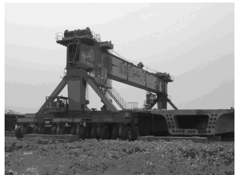
图12 单立柱单主梁900 t轮胎式搬梁机 Fig. 12 900 t wheel girder mover of single pillar and single girder
