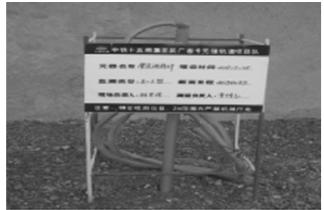
图12 埋设后的单点沉降计 Fig.12 installed settlement sensor
