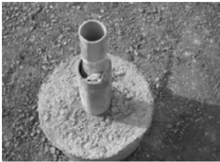
图9 沉降板示意图 Fig.9 Settlement plate
