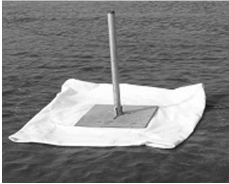
图9 沉降板示意图 Fig.9 Settlement plate
