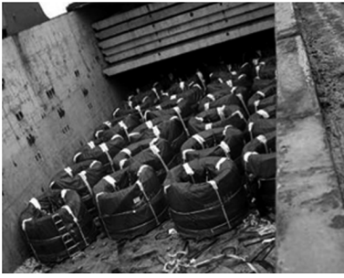
图7 货物规则摆放 Fig. 7 Regularly put cables
