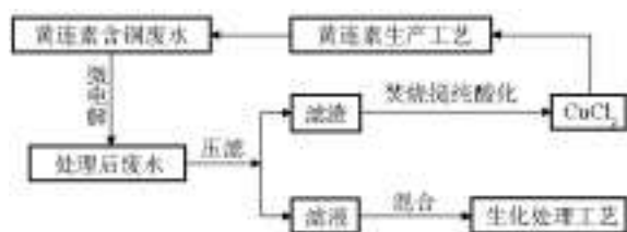
图8 黄连素含铜废水处理及铜回收工艺流程 Fig.8 Process of wastewater treatment and copper recovery
