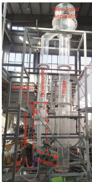
Fig. 8. Schematic diagram of an external loop slurry reactor integrating mixing and separation.
