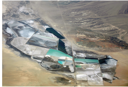
Fig. 2. The Albemarle Corporation lithium operation near Silver Peak, NV, USA, covers more than 5200 hm 2 and uses brine pumped from underground to produce lithium carbonate through evaporation. The process takes up to 24 months to complete. Credit: Doc Searls (CC BY 2.0).
