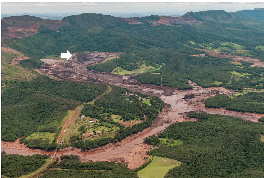
**Fig. 1.** In one of the deadliest tailings dam disasters in history, the 25 January 2019 collapse of the tailings dam (arrow) at the Córrego do Feijão iron ore mine near Brumadinho, Brazil, sent a wave of toxic mud downstream, killing 237 people and destroying 269.84 hm<sup>2</sup> of land. Credit: Vinícius Mendonça/Ibama (CC-BY-SA-2.0).
