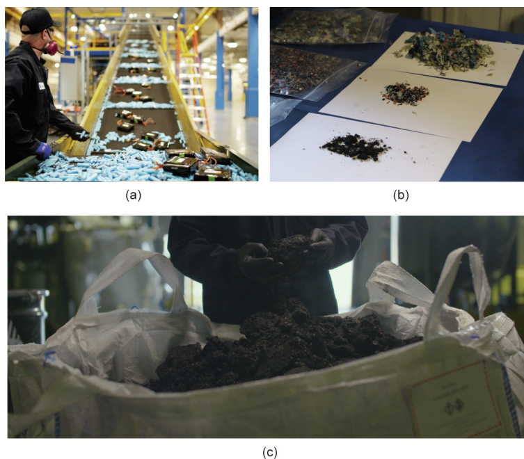
Fig. 2. (a) LIB of various kinds—though no EV batteries in this picture—cascade down a conveyor belt for processing at Li-Cycle’s Rochester, NY, USA, “Spoke” facility. (b) Once shredded, the battery materials are sorted into plastics (top), aluminium/copper foils (middle), and the anode/cathode materials, known as “black mass” (bottom). (c) The black mass is collected for recycling of its nickel and cobalt content by hydrometallurgical reclamation. Credit: Li-Cycle, with permission.
