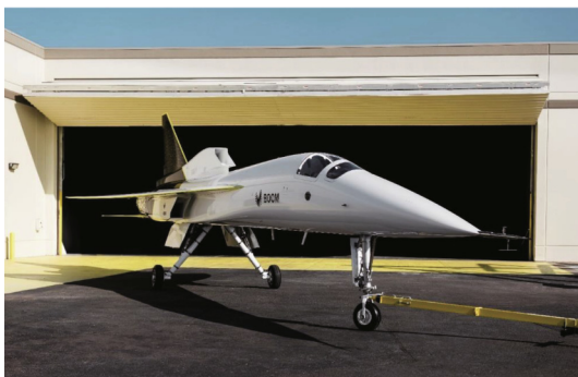
Fig. 1. Boom Supersonic’s XB-1 prototype aircraft, unveiled in October 2020, is a one-third-scale version of its planned Overture commercial SST. Credit: Boom Supersonic (public domain).
