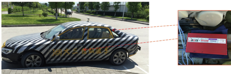
Fig. 7. The prototype car equipped with an inertia sensor.
