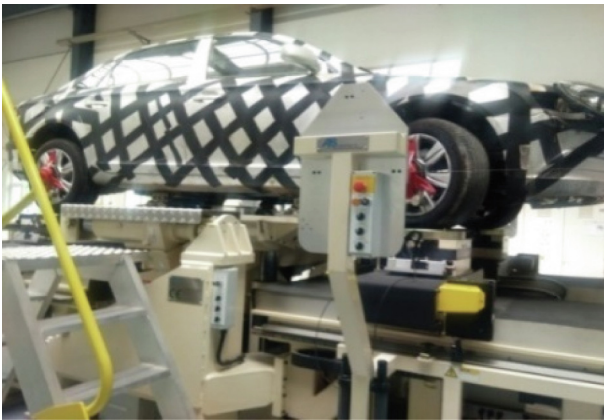
Fig. 6. The prototype car during the K&C test.
