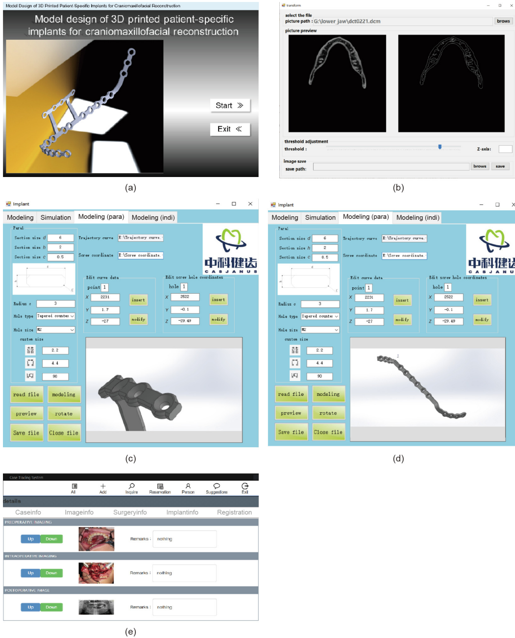
Fig. 2. Our design module, which was developed on Solidworks®, will help surgeons to design the patient-specific implant. (a) The interface of our design module; (b) read a 3D CT model; (c) specify the cross-section of the implant; (d) use point-and-pick key points to generate the implant design; (e) generate a patient-specific implant record.
