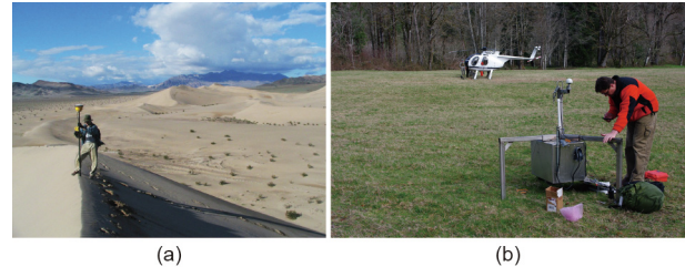
Fig. 11. (a) A Smithsonian Institution researcher uses a high-precision GPS device to survey a sand dune in 2005 at Ibex Dunes in Death Valley National Park in California, USA. (b) A US Geological Survey (USGS) team sets up a portable “spider” instrumentation package containing high-precision GPS units to monitor movement in a March 2014 landslide in northwest Washington, USA. Credits: Jim Zimbelman, National Air and Space Museum, Smithsonian Institution (public domain); Jonathan Godt, USGS (public domain).
