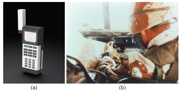
Fig. 1. Sent to US troops in the Middle East by their families back home, GPS receivers made for civilian use, such as (a) the 1991 Magellan NAV 1000 and (b) the Trimble Trimpack mounted in a military vehicle, provided unprecedented navigation guidance in the Desert Storm campaign. Credits: The Science Museum (CC0); US Army (public domain).
