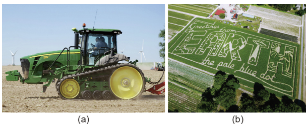
Fig. 10. (a) A Starfire(D) GPS receiver installed at the canopy front of this John Deere 8345 RT tractor guides its satellite-assisted steering system. (b) Guided by precision GPS, Precision Mazes (Lee’s Summit, Mo, USA) created this corn maze in Sunderland, MA, USA. Credits: bdk, Wikimedia Commons (CC BY-SA 3.0); Precision Mazes (public domain).
