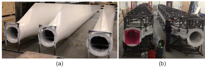
Fig. 8. Advanced materials for turbine blades. (a) 13 m single-piece wind blades for 250 kW turbines; (b) these are produced from glass/carbon fiber and powdered epoxy resins using electrically heated ceramic composite tooling (photographs courtesy of Prof. Conchúr Ó Brádaigh and ÉireComposites).
