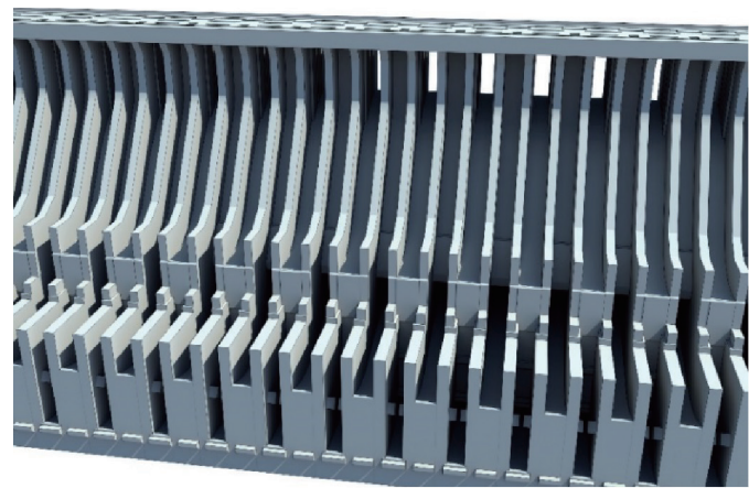
Fig. 3. Three-dimensional diagram of the three-layer orifices.
