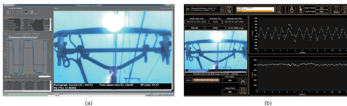
Fig. 9. (a) Arc measurement results of the HEMU-430X at 400 km·h -1 ; (b) dynamic stagger/height measurement results of the HEMU-430X at 400 km·h -1 .
