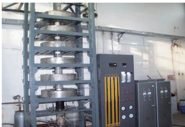
Fig. 6. Experimental apparatus of the magnetically stabilized bed reactor.
