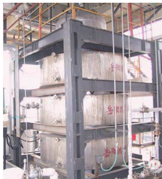
Fig. 8. The 100 kt·a -1 CPL purification magnetically stabilized bed reactor unit.
