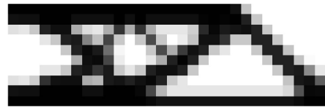
Fig. 4. The topology optimization result.
