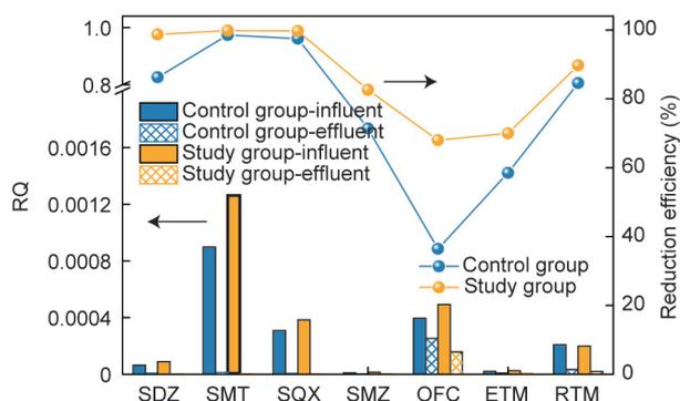
Fig. 3. RQs in influent and effluent and corresponding reduction efficiencies in the control group and study group of the investigated DWTPs (age interval of 0–3 months).
