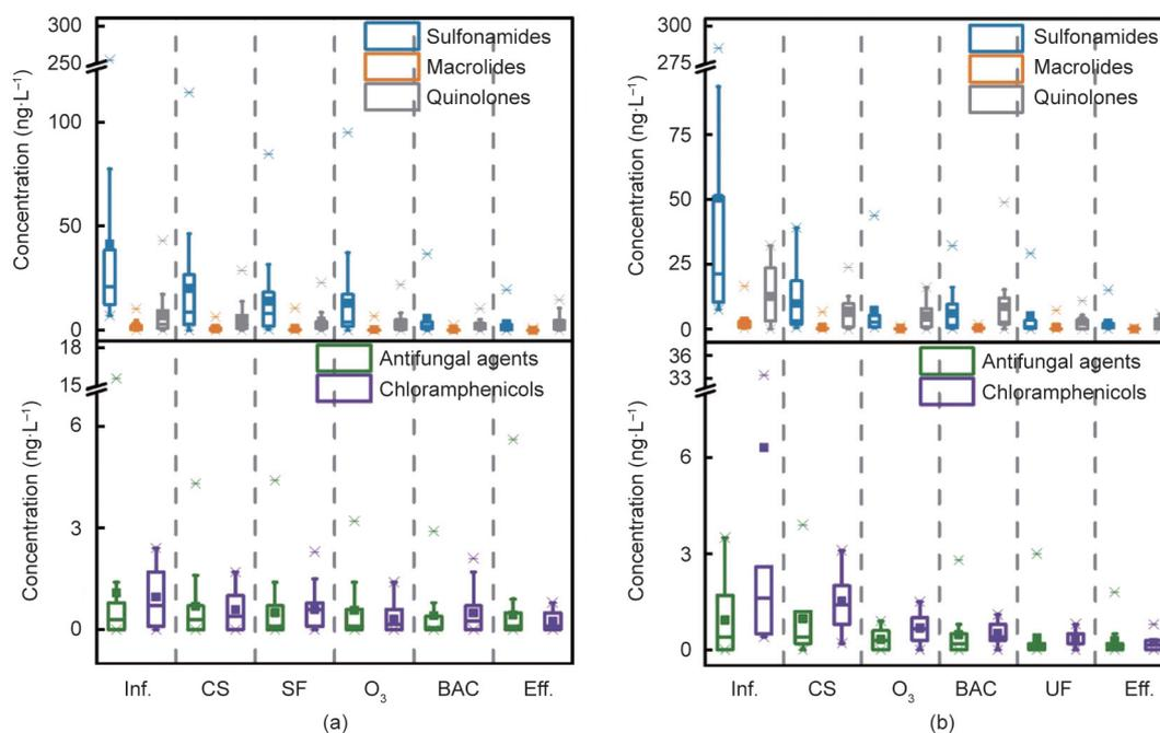
Fig. 2. Variations in antibiotic concentrations after each process in (a) DWTPs in the control group and (b) DWTPs in the study group.
