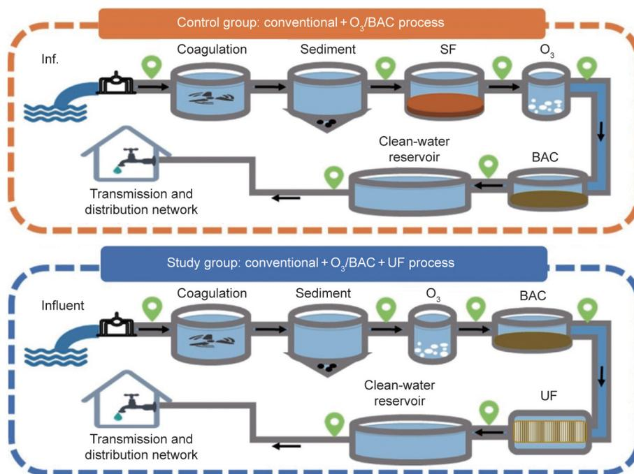
Fig. 1. Schematic diagram of the treatment processes of the investigated DWTPs.
