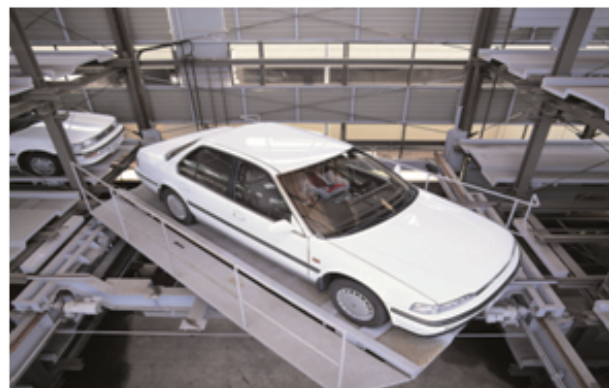
Fig. 7. Lift-sliding mechanical parking system.
