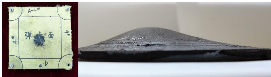
Fig. 7. Target plate and the steel back plate of the gradient B 4 C/Al composite after the projectile.
