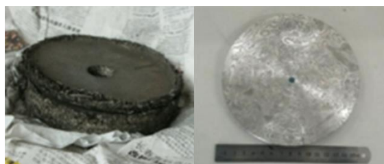
Fig. 8. C f /Mg composite disc samples (after high speed centrifugal test).
