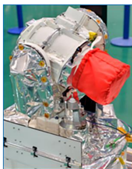
Fig. 3. Space motion optical system made of SiC/Al composites.
