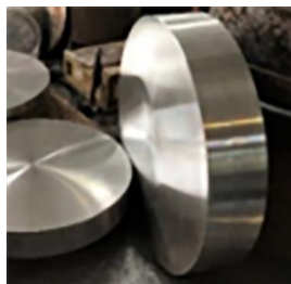
Fig. 2. \phi 900 mm instrument-grade SiC/Al composite embryo.
