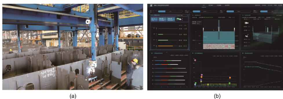
Fig. 7. Immersed tube factory production in Shenzhong channel using (a) an intelligent production line and (b) an intelligent quality control system.
