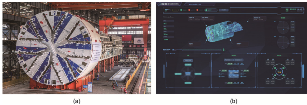
Fig. 6. (a) An intelligent shield machine and (b) a shield control system platform developed by the Shanghai Tunnel Engineering Co., Ltd.
