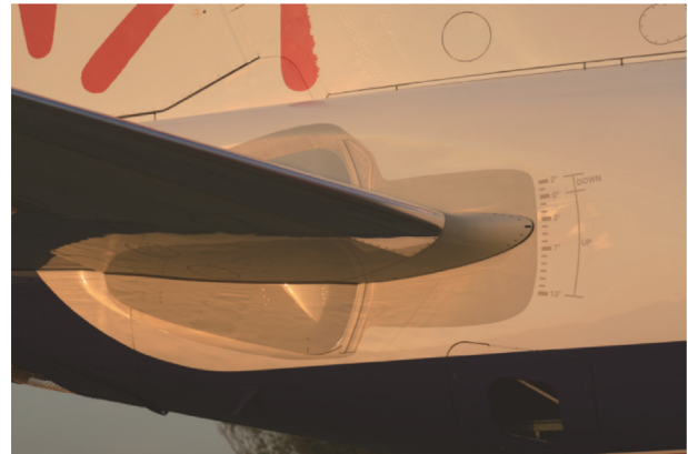
Fig. 1. In certain situations, the MCAS of the Boeing 737 Max 8 was designed to automatically move the horizontal stabilizer, like this one on the Embraer ERJ-170, to push the nose of the aircraft down to prevent stalling. Credit: YSSYGuy, English Wikipedia (CC BY-SA 3.0).
