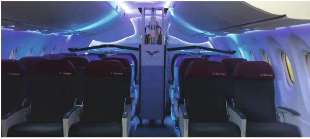
Fig. 2. The GermFalcon is a UV disinfection device that can be wheeled up and down an airplane aisle. It requires an operator, who is protected by a UV light shield, to push it. Credit: Dimer UVC Innovations, with permission.
