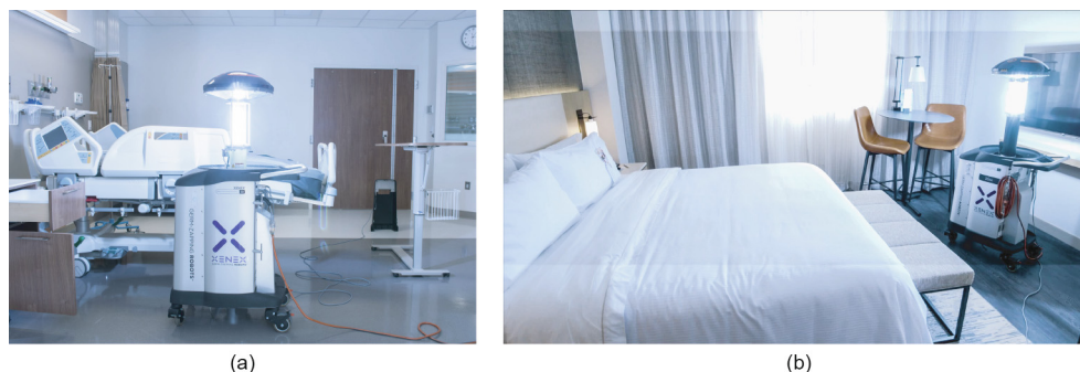
Fig. 1. The Xenex LightStrike, shown here set up inside (a) a hospital room and (b) a hotel room, is stationary during use, but the “head” moves up and down, and its xenon lamp pulses many times a second with UV light that spans the spectrum from 200 to 315 nm. Credit: Xenex, with permission.
