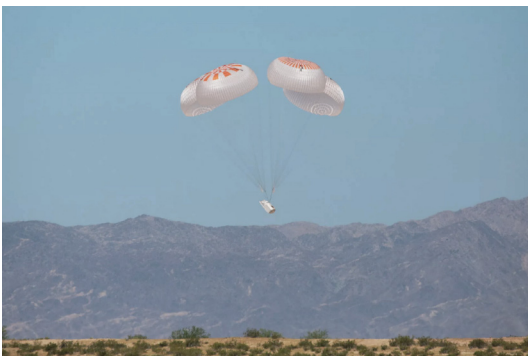
Fig. 3. The Crew Dragon uses a four-piece parachute system, shown here in a test, to bring the capsule gently back to Earth. Credit: SpaceX (public domain).
