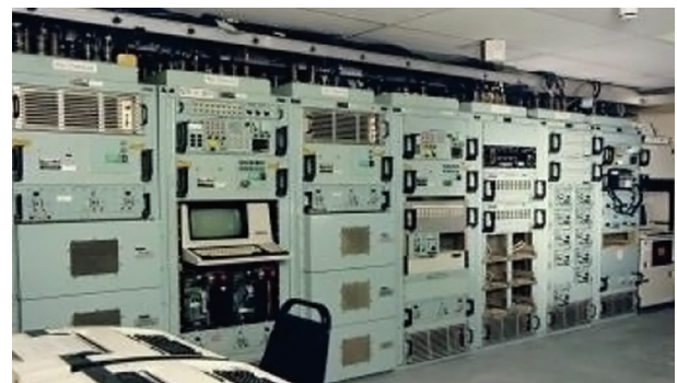
Fig. 1. The US Department of Defense uses an IBM Series/1 computer from the 1970s to help control the country's nuclear arsenal. Until 2019, the computer still needed 8 in floppy disks. Credit: US GAO (public domain).
