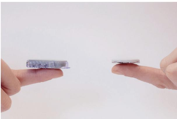
**Fig. 2.** Dexcom's G7 sensor (right) is 60% smaller than its predecessor, the G6 (left), but still larger than the FreeStyle Libre 3. While the G7 and Abbott FreeStyle Libre 3 are expected to gain approval for this application, the G6 is currently approved for use, integrated with Tandem's X2 insulin pump, as part of a closed-loop, automated insulin delivery system. Credit: Dexcom (public domain).
