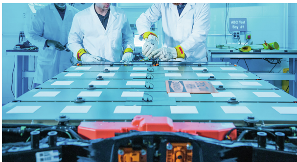
Fig. 1. Beneath the cover plates forming the uncluttered surface of this high-voltage EV battery pack in the GM Battery Electrical Laboratory in February 2020, multiple battery modules enclose close-packed electrochemical cells. The modules wirelessly communicate with each other and the vehicle's microprocessor-based battery monitoring system, an advance co-developed by GM and electronics maker ADI. Credit: Jeffrey Sauger/GM (public domain).
