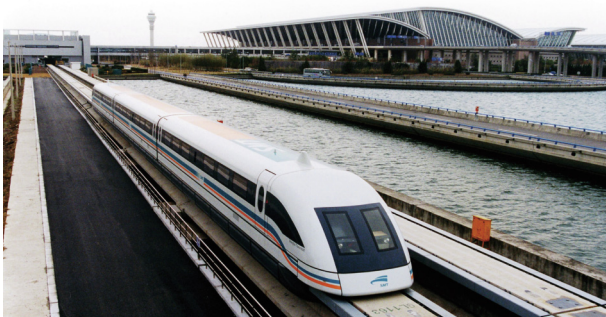
Fig. 1. Running at a top speed of 431 km·h -1 , the world's longest and oldest maglev line spans the 30 km stretch between Shanghai's Pudong Airport and Longyang Road on the eastern side of the city. Credit: Alex Needham (public domain).
