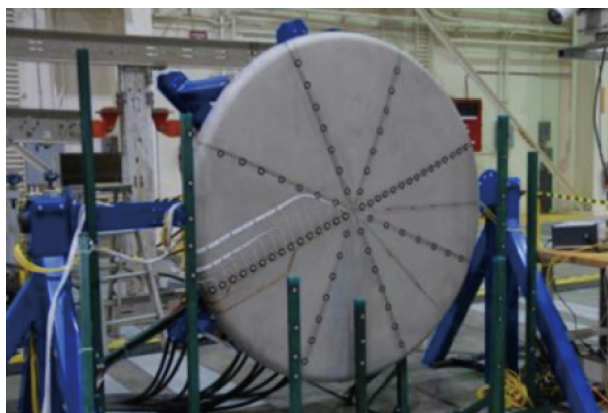
Fig. 8. Experimental verification of the FOSS monitoring of the spacecraft thermal protection structure, jointly carried out by NASA and CSIROO [30,31].
