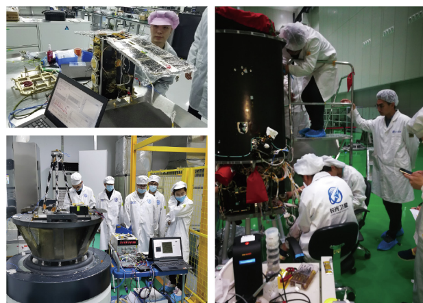
Fig. 10. A series of flight verification tests for optical fiber sensing systems on various types of satellites carried out by BISTU.
