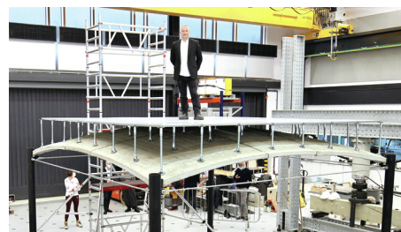
Fig. 2. Designed by Paul Shepherd of the University of Bath in the United Kingdom and colleagues, this curved concrete slab generates 60% less greenhouse gas emissions than a traditional slab. Shepherd is standing atop a floor resting on the slab. Credit: University of Bath, with permission.
