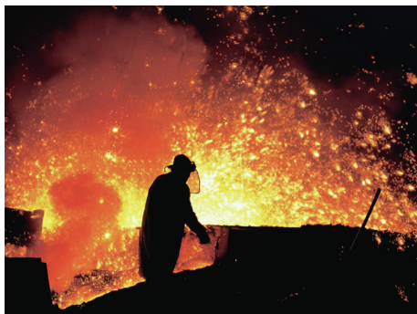
Fig. 3. Amid this shower of sparks from a steel plant's blast furnace, iron ore and coking coal are reacting to produce pig iron and CO 2 . In the most common steel-making process, this step yields the most CO 2 . Credit: Třinecké železářny, with permission.
