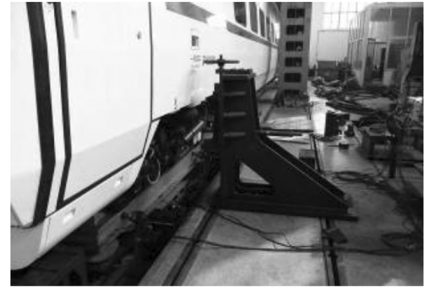
图7 CRH5动车组悬挂参数测定试验 Fig. 7 Measuring suspension parameters of EMU CRH5
