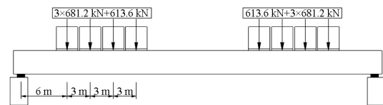
图7 节段加载工况 Fig.7 Segment loading cases
