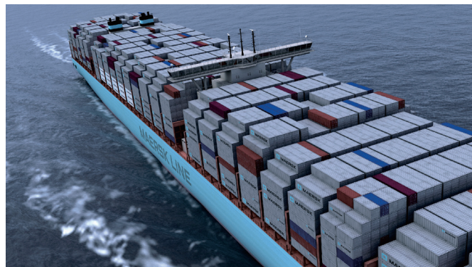
Figure 3. The Triple E. An example of the new generation of large container ships; it is 400 m long and 59 m wide, has a speed of 19 kn and carries 165 000 DWT. ( http://www.maersk.com/en/search?q=Triple%20e&t=images , 12 February 2015)
