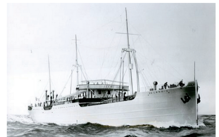
Figure 1. MS Selandia . The first ocean-going diesel motor ship, carrying 6800 DWT, built by B&W in 1912 and assigned to the EAC. ( http://selandia100.dk/diesel-2 , 12 February 2015)
