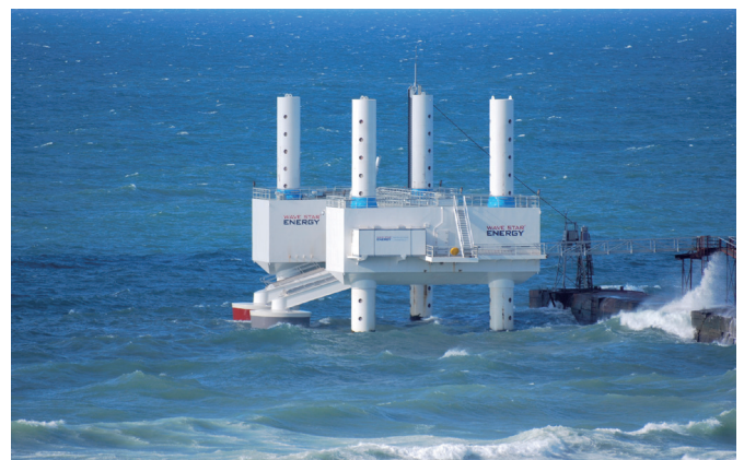
Figure 10. A 1 : 2 scale jack-up structure that draws energy from the waves by means of floating point absorbers. (Permission by Wave Star A/S)
