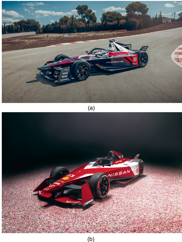
Fig. 2. The third-generation Formula E racers from (a) Porsche and (b) Nissan look alike because all cars in the competition have the same body design, maximum power, and battery capacity. What sets Formula E teams apart is the design of their powertrains, their strategies for managing battery power, and the skill of their drivers. Credit: (a) Porsche (public domain); (b) Nissan (public domain).
