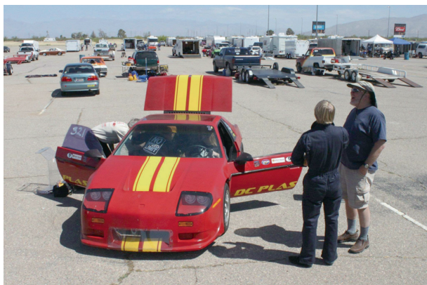
Fig. 1. John Metric upgraded this Pontiac Fiero by adding two electric motors where the gas tank had been and installing a 375 V lithium-polymer battery pack. The vehicle set an electric racing record for its class by covering the 1/4 mile (0.4 km) in 9.898 s. Credit: John Metric, with permission.
