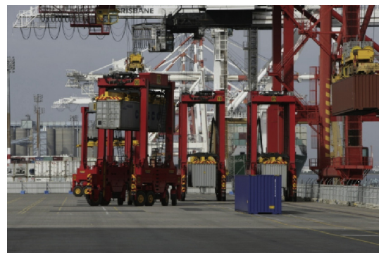
Fig. 1. Fully autonomous straddle carriers operating in the port of Brisbane, Australia.
