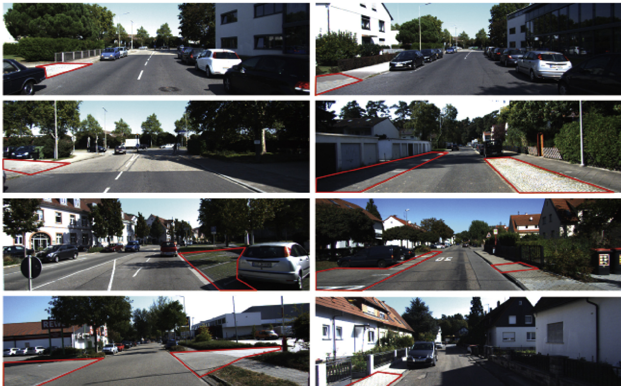
Fig. 11. Examples of areas with ambiguous semantics. The image areas bounded by red lines are not “road” in a narrow sense, but many of these areas are designed for driving.
