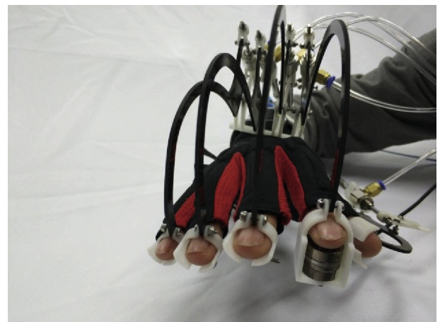
Fig. 14. The physical prototype of the measurement device.
