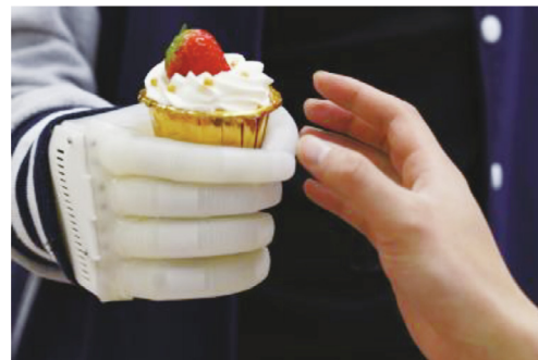
Fig. 1. A soft, elastic, lightweight robotic hand engineering to provide simultaneous myoelectric control and tactile feedback gives amputees greater control than traditional neuroprosthetic hands [6]. Credit: Massachusetts Institute of Technology/Xuanhe Zhao (public domain).
