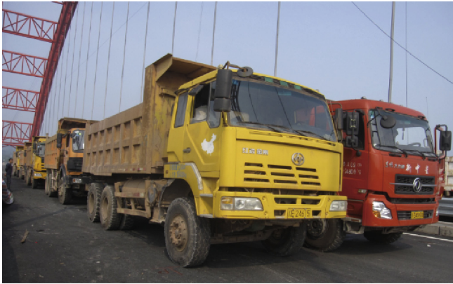
Fig. 13. The load test of the First Hejiang Yangtze River Bridge after completion.
