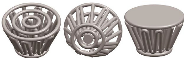
Fig. 1. The structural diagram of the new tubular airbag.
