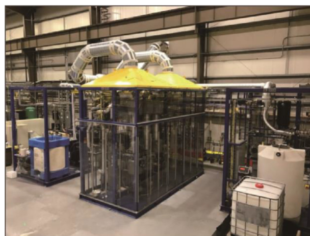
Fig. 1. A skid-mountable HTL unit developed at PNNL. The carboy pictured at front right has a volume of about 1 m 3 .
