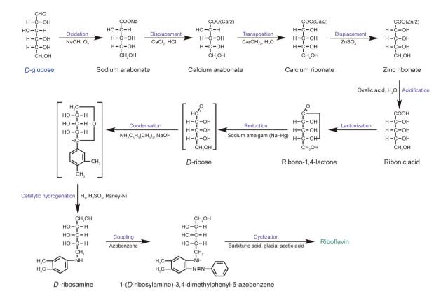
Fig. 2. The total chemical synthesis of riboflavin.
