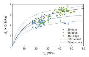
**Fig. 6.** Relation of elastic modulus and peak stress. The dotted line means the 95% confidence interval. Reproduced from Ref. [16] with permission.
