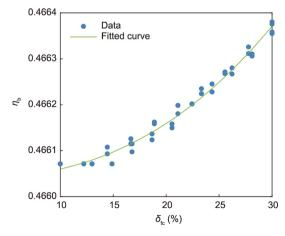
Fig. 10. Minimum reinforcement ratio coefficient of RAC beams.
