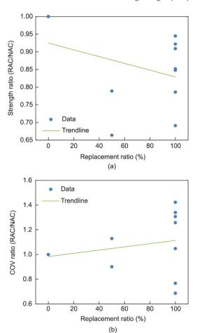
**Fig. 2.** The relationship between the replacement ratio and (a) the tensile strength ratio and (b) the COV ratio (RAC/NAC).
