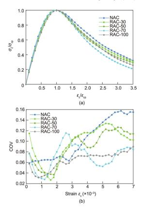
**Fig. 4.** (a) The normalized stress–strain curve and (b) the relationship between the COV and strain of the NAC and RAC with different replacement ratios.  $\sigma_c$ : compressive stress;  $\sigma_{cp}$ : peak compressive stress;  $\varepsilon_c$ : compressive strain;  $\varepsilon_{cp}$ : peak compressive strain. The number following RAC (30, 50, 70, 100) means the replacement ratio of RAC in percentage.
