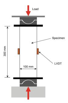
Fig. 3. Loading device. LVDT: linear variable differential transformer.
