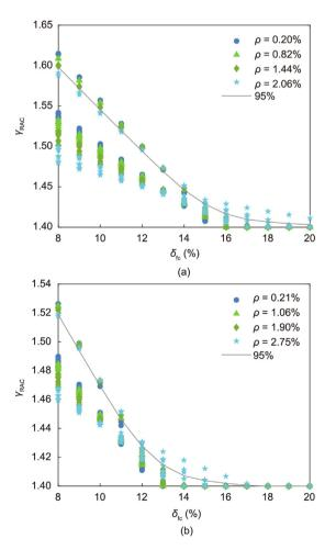
**Fig. 9.** Partial safety factors of RAC: (a) C30 and (b) C40.  $\gamma_{RAC}$ : partial safety factor of RAC;  $\delta_{fc}$ : COV of compressive strength.
