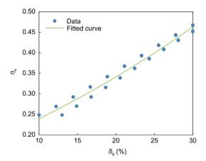
Fig. 11. Minimum stirrup ratio coefficient of RAC beams,  $\delta_{\rm ft}$ : COV of the tensile strength.
