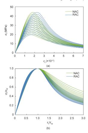
**Fig. 8.** Comparison of NAC and RAC at different strength levels: the main stress-strain curves (a) with and (b) without normalized.
